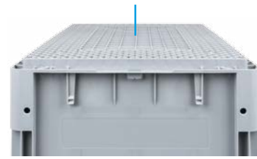
Reinforced bottom with 45° ribbed perimeterband and 90° ribbed central part for bending compensation
